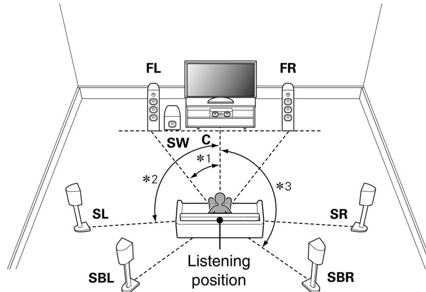
Figure 2: Layout of a standard 7.1 channel surround sound system. The angle values are as follows: Angle 1 = 22° to 30°, Angle 2 = 90° to 110°, Angle 3 = 135° to 150°.
