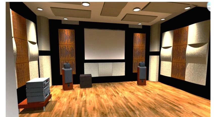
Figure 5: Example of room treatment in a home theater system. The white panels on the right and left of the room are sound absorbing panels. The wooden panels with slits in them are also sound absorbers. There are also sound absorbers on the ceiling. There are four bass traps, two per corner.
